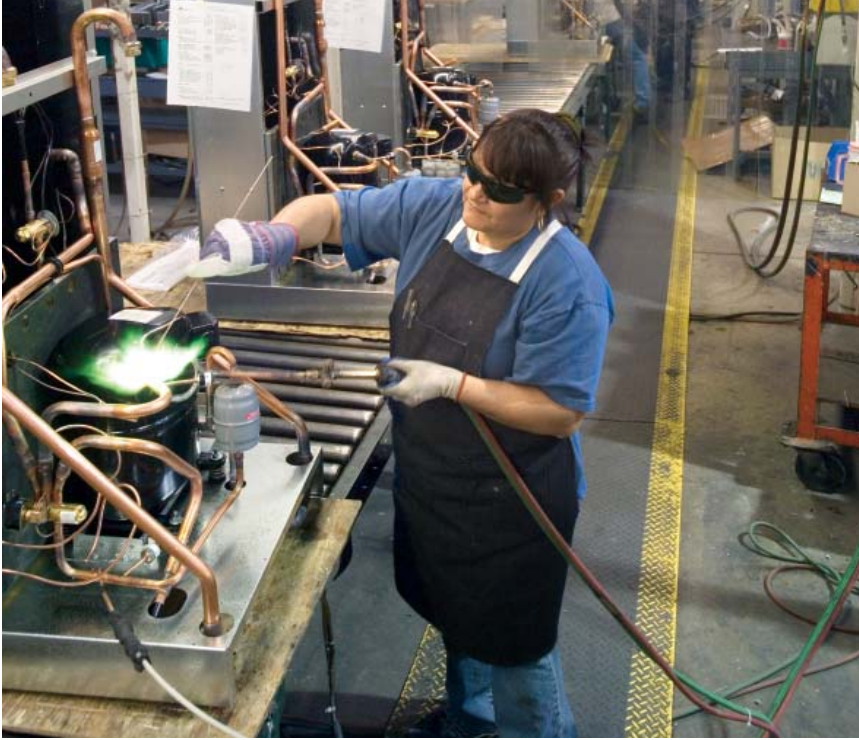
ClimateMaster employee brazing in components.
